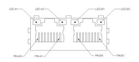
On the connectors there are also two LEDs for each port. Left LED is bicolor (Green /Yellow) and shows 10/100 or 1000 connection: green means 100Mbps connection, yellow means 1000Mpbs connection, when the LED is Off then 10Mpbs or no connection is available. The right LED is Green and shows ACTIVITY presence.
