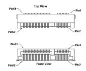
Due to the reduced dimensions of the board itself, on the SBC-992-pITX board it is only possible to insert Half-Size miniPCI express cards.
