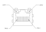
Both connectors are RJ-45 sockets type LINK-PP p/n LPJG16314A4NL or equivalent, with 2kV decoupling capacitor, 100 Ohm impedance.
